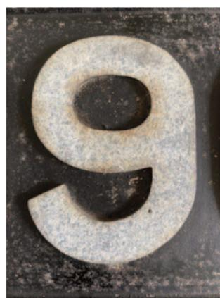
Favourite Digits, is very well thought out as the base plate is cast with a pattern of dimples on the back in each of the location rectangles for the characters to be used. The characters had small 'pins' cast on their reverse which, depending on which character is needed to construct any particular mark, dictates which dimple is to be used. The centre for a small hole which is drilled and the character fitted by
