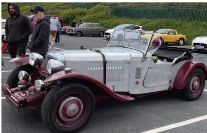
On investigation it turned out to be a TA14 chassis, wheels and radiator but not much else! The owner had battered the wings out of some steel he had lying around using what sounded like a hammer and a piece of wood and had made a pretty good fist of it. The car had an MGB engine and gearbox as the owner wanted something he could swap out easily when it failed - he clearly didn't understand Alvis' legendary reliability. Either that or he had no faith in his spannering skills
